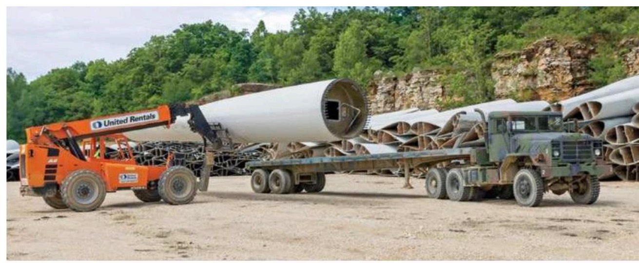
Partially disassembled wind turbine blades arrive at Veolia North America's recycling facility in Missouri, where workers offload the decommissioned blades (left) and cut them (middle) for shredding. Veolia sends the shredded material (right) to customers who blend it with raw materials to make cement.
